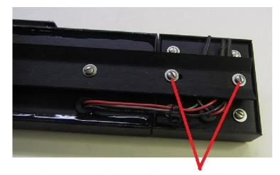
Remove these 2 screws to access programming switches
